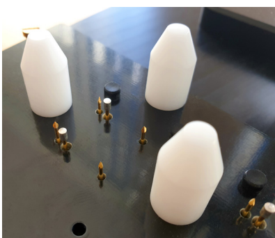
Figure 6: 1000A pulse with one needle per contact.
