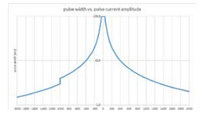
The integrated "Ixt limiter" provides a multitude of current -pulse length combinations while monitoring the maximum currenttime product.
